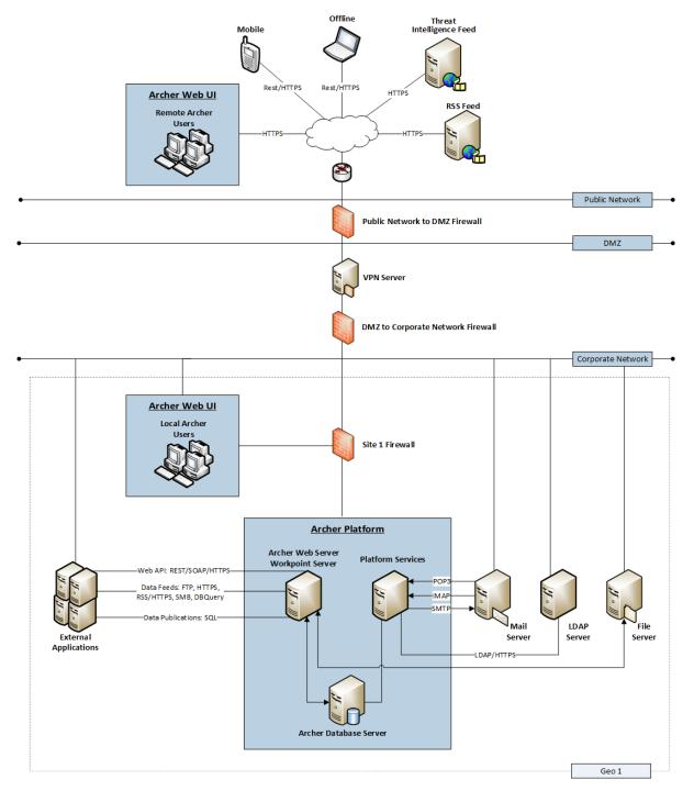
The following figure shows an example of a multi-host configuration.
